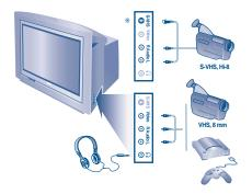
Carry out the connections featured opposite. Using the key, select EXT3 for a VHS or 8mm camcorder and S-VHS3 for an S-VHS or Hi-8 camcorder.
