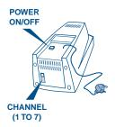
3 At the bottom of the active loudspeaker, set the slide channel to channel 1. Switch on the active speaker with the power switch. The indicator at the front of the active speaker lights up red when the speaker is in standby and green when there is a surround sound transmission. It turns back to red (standby) when the tv is switched off or when the rear channel is not used (in the case of STEREO, DOLBY 3 STEREO and 3D SURROUND modes).
