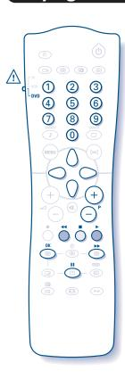
A First you must switch the mode selector located on the side of the remote control to the DVD position.
