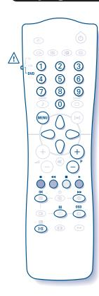
⚠ To access the DVD functions you must first switch the mode selector located on the side of the remote control to the DVD position.
